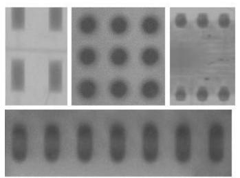
Figure 5. X-ray images of lead-free solder.
